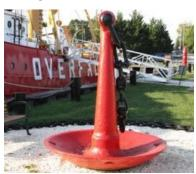
edge are designed to help break the suction on the anchor when it is being retrieved.
